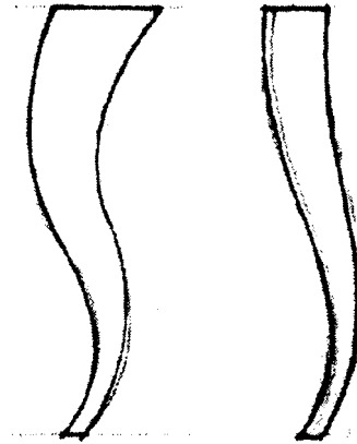
Fig. 2. Curve of leg made with French curve (left) vs. leg made with wood strip (right).
